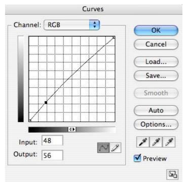
The adjustment curve I used for images printed on the R260 to compensate for a slightly darker print quality than on the R800 or on my Epson K3 Printers.
